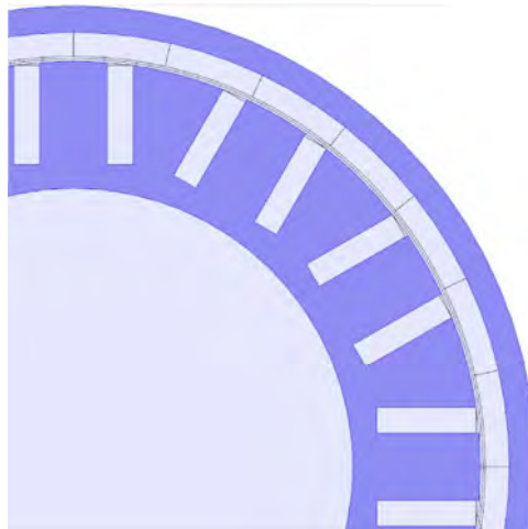
Figure 3.12: Geometry of synchronous machine 24 slots 28 poles with maximised EMF.
